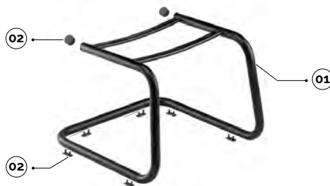
01 sl43-base coulissante tube ø30 embouts exclus sl43-base patin tubular ø30 tapones excluidos
